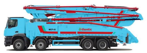
The Atlantic MCP 43 is a high-performance truck-mounted concrete boom pump engineered for maximum efficiency, reliability, and precision on demanding job sites. Assembled on a standard 4-axle chassis, the MCP 43 features a robust 43-meter, 5-section, RZ-type placing boom developed using advanced FEM design techniques for optimal strength and flexibility.
